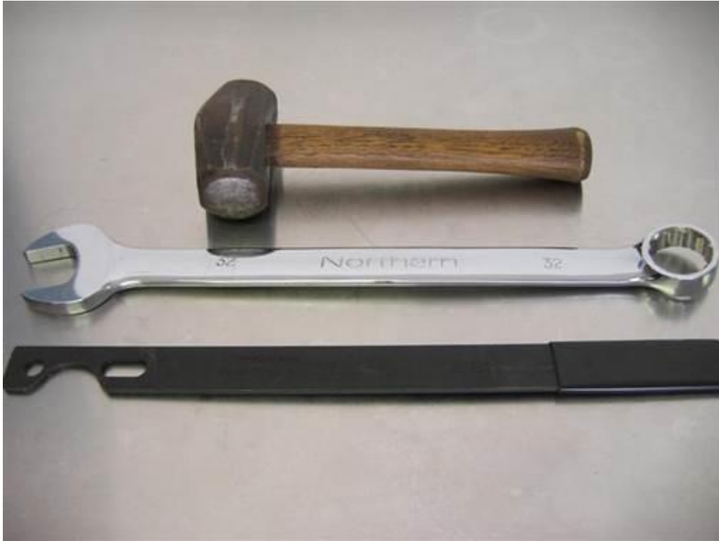
E36 & E39 mechanical fan removal tools 32mm combo wrench, BMW water pump pulley holder (11-5-030) $20/each Handheld sledge hammer (3lb)
