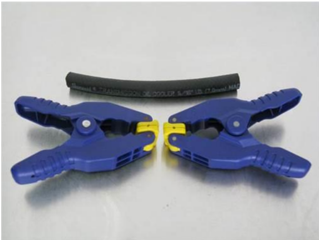
E36 fan/shroud removal tools ~6" x 5/16" (8mm) vacuum hose, 2 small clamps
